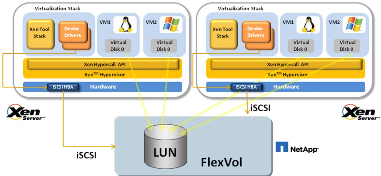
Figure 5 Shared iSCSI storage using iSCSI HBA
