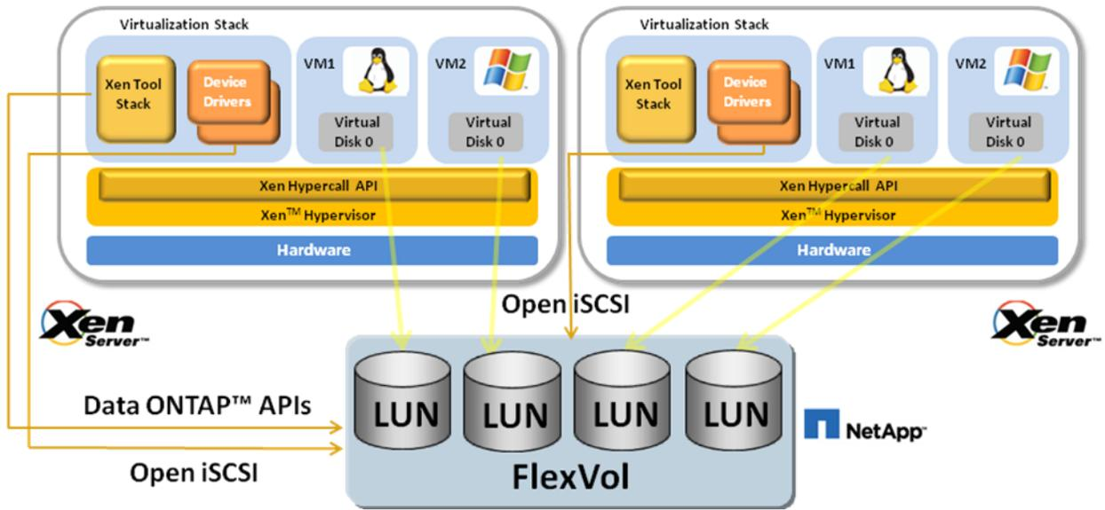
Figure 2 Shared storage using NetApp Data ONTAP
