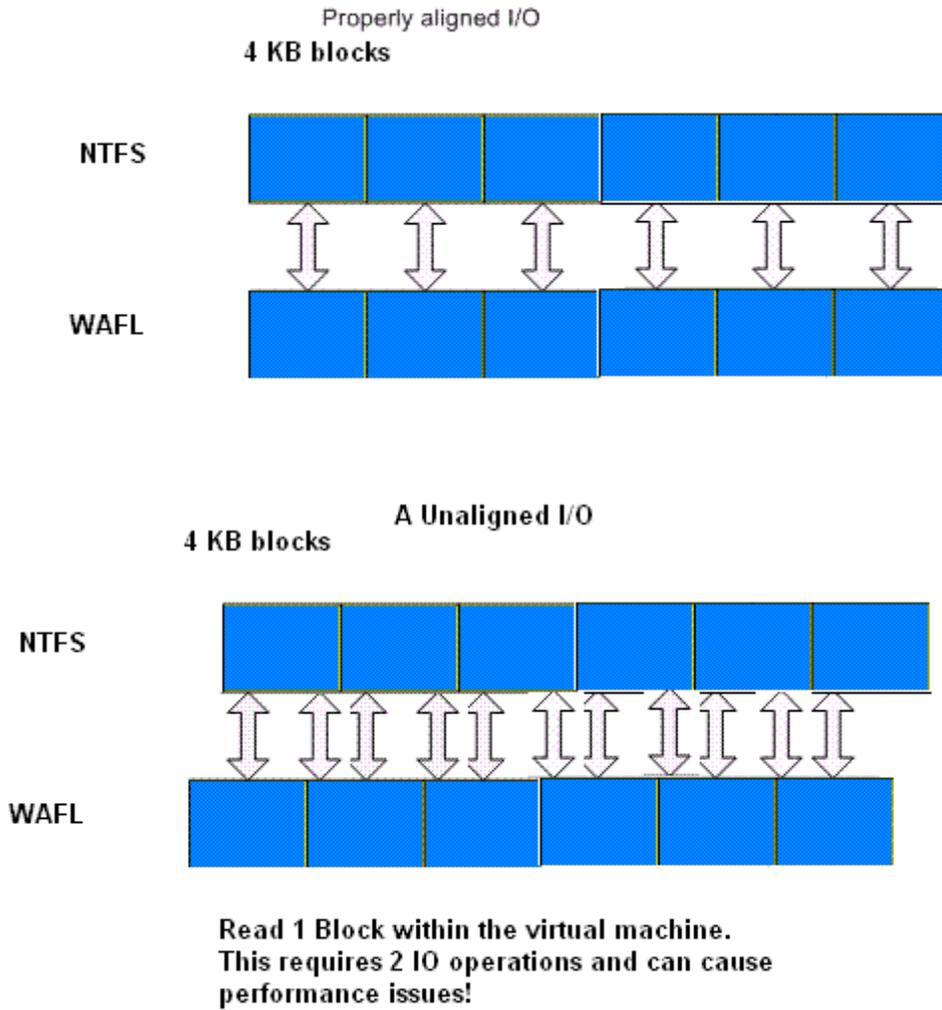
Figure 9 Properly aligned and unaligned I/O.
