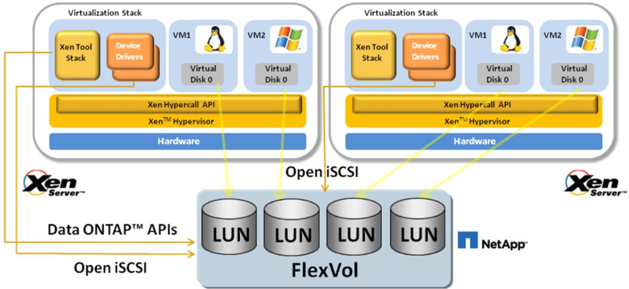
Figure 2 Shared storage using NetApp Data ONTAP
