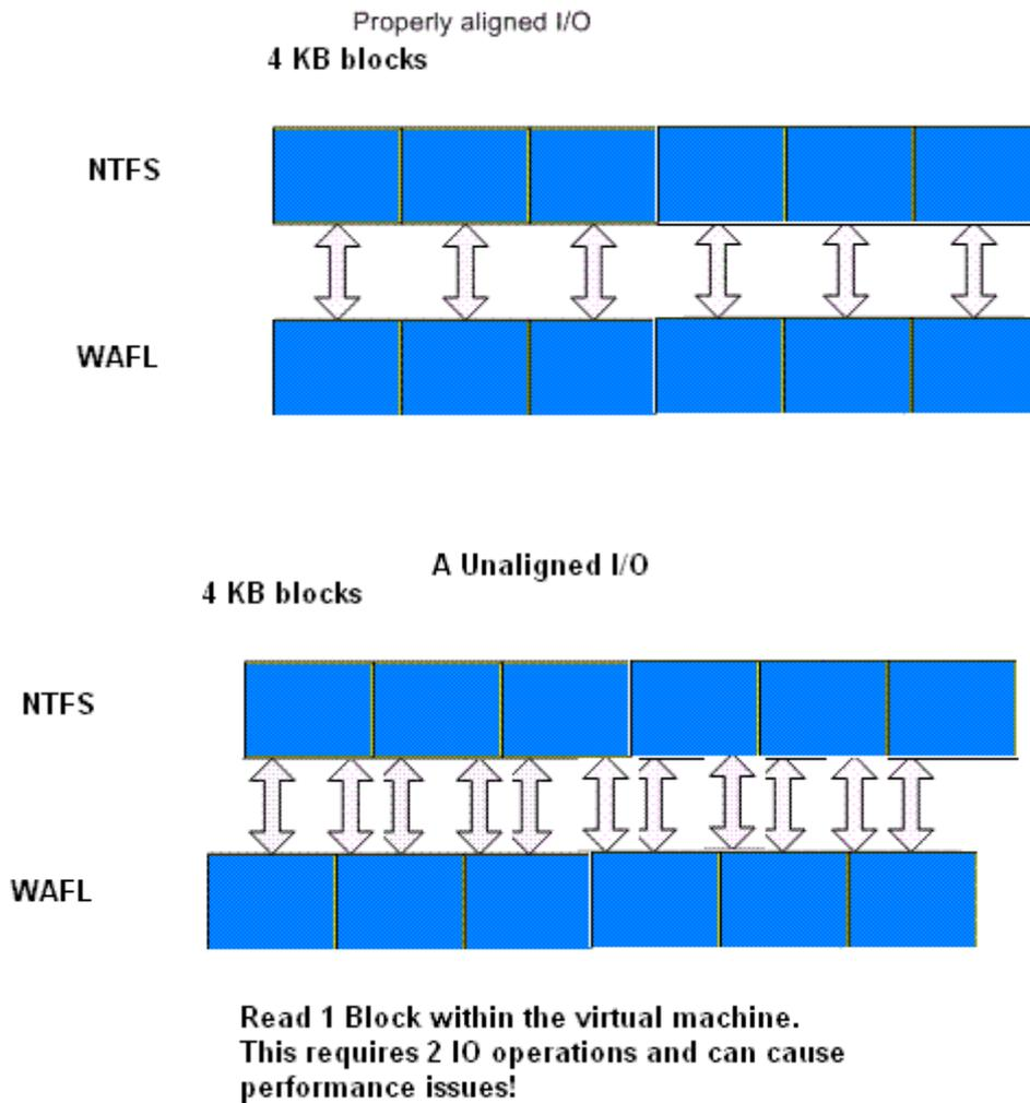
Figure 9 Properly aligned and unaligned I/O.
