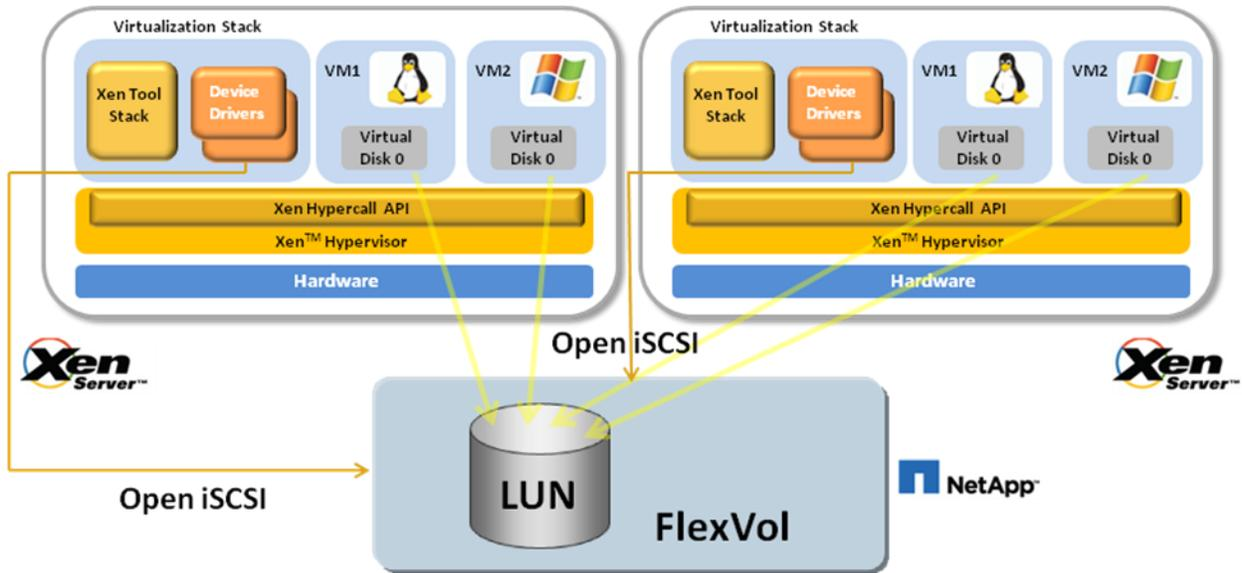
Figure 4 Shared iSCSI storage using Open iSCSI initiator
