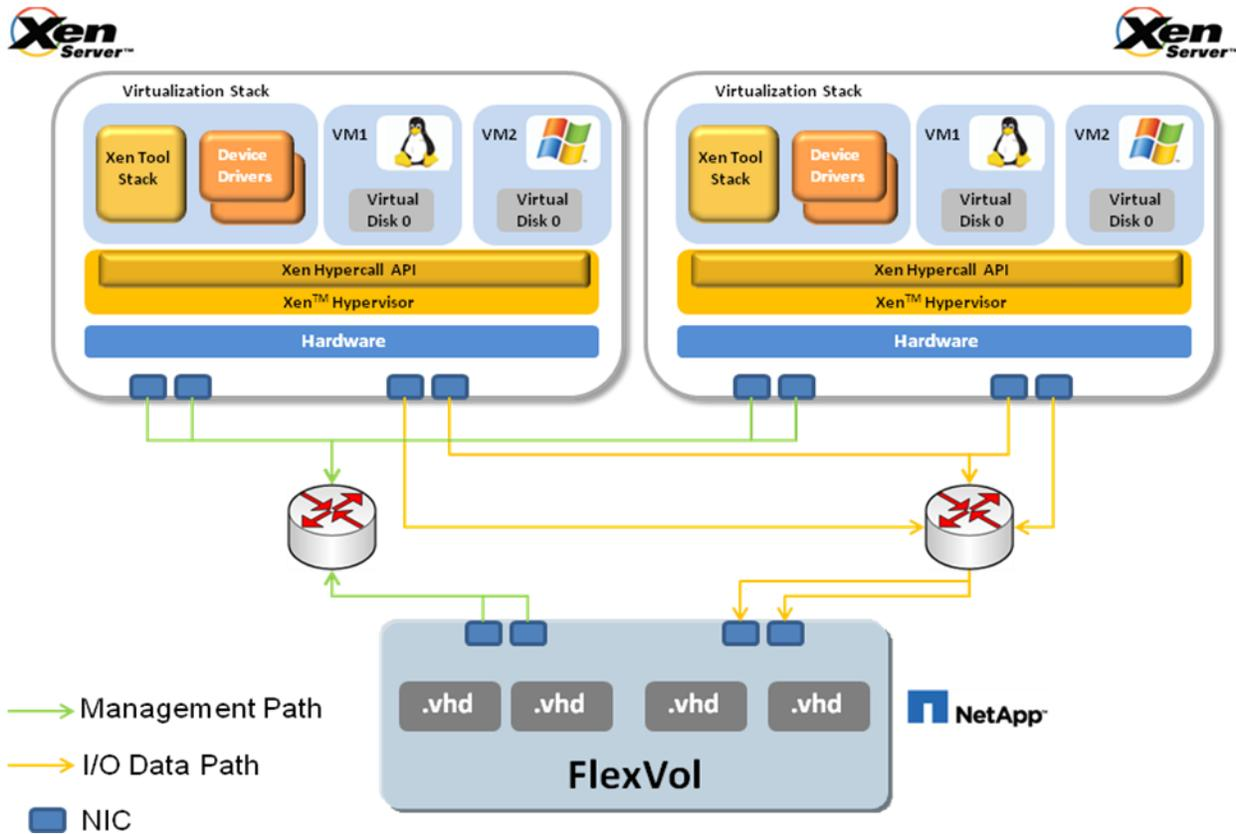
Figure 8 Graphical representation of NIC bonding configuration
